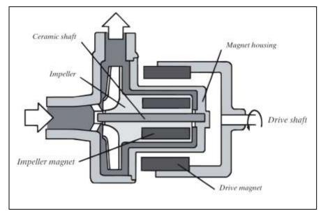
*Mag-Drive* drive pumps are capable of pumping a variety of liquids. Some devices are designed to move Abrasive Materials, Acids, Adhesives, Chemicals, Concrete and Grout, Coolants, Hazardous Materials, Liquid Metal, or Lubricants.
